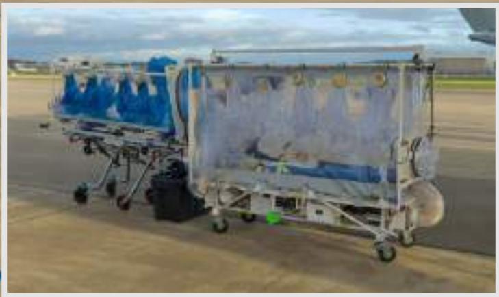
This Air Transportable Isolator (ATI) system is used specifically by aeromedical isolation teams to initially transport and transfer infected patients safely to larger hospital isolation units. The envelope holds a stretcher and therapeutic equipment which allows medics to care for the patient throughout the transportation phase of their treatment.
