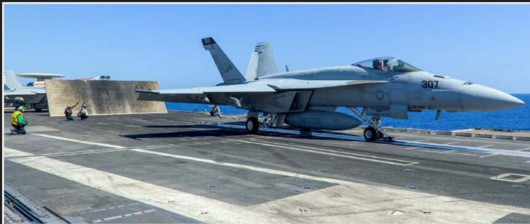
The catapult shuttle accelerates an F/A-18 to 150 - 160 kts within about three seconds.
