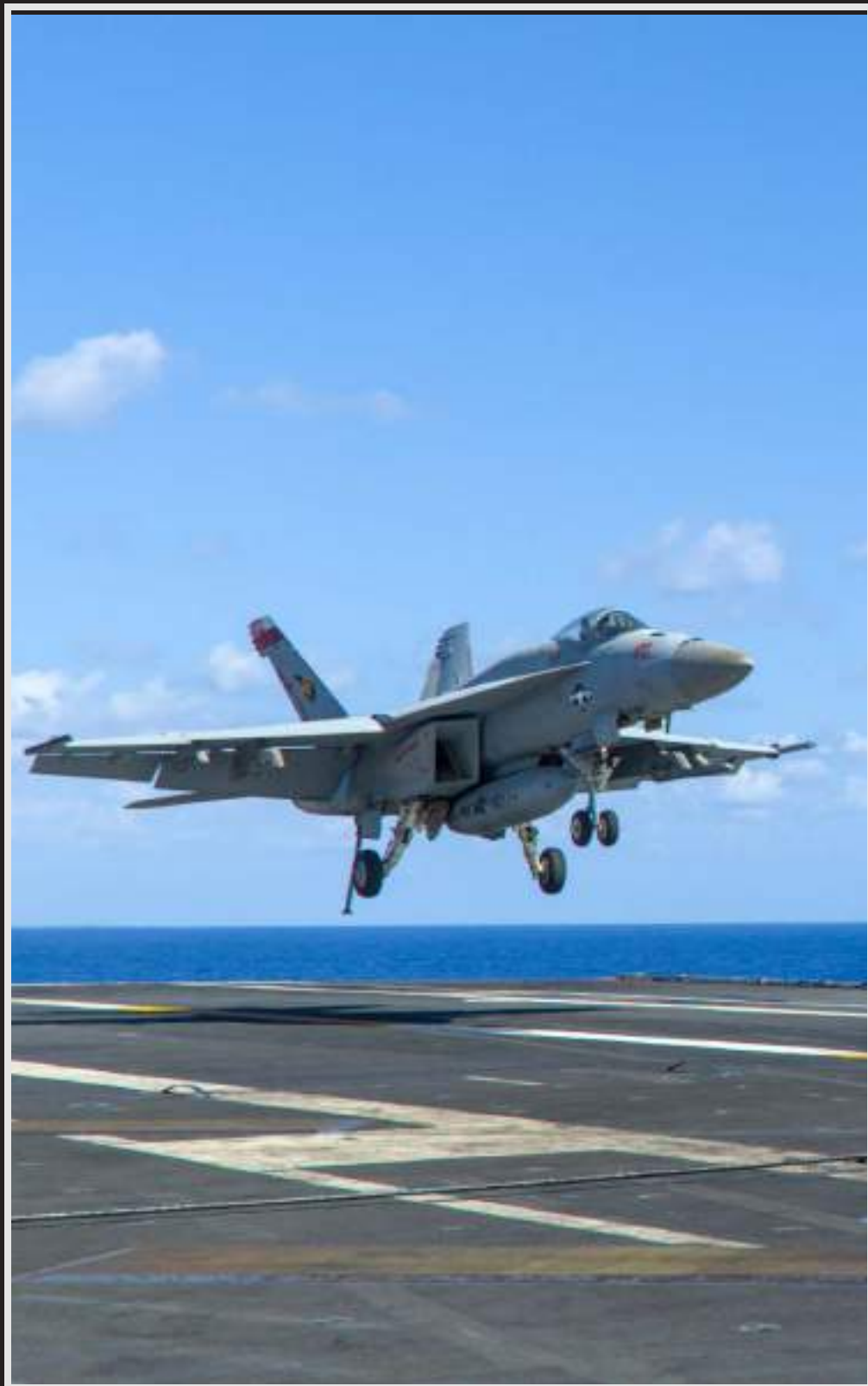
There are only two arresting cables in use, with one spare arresting installation. On most Nimitz-class carriers, there are four wires across the deck (pilots are aiming for the third wire during landing). The last carrier of the Nimitz-class, the USS Bush, only had three arresting cables across the deck.
